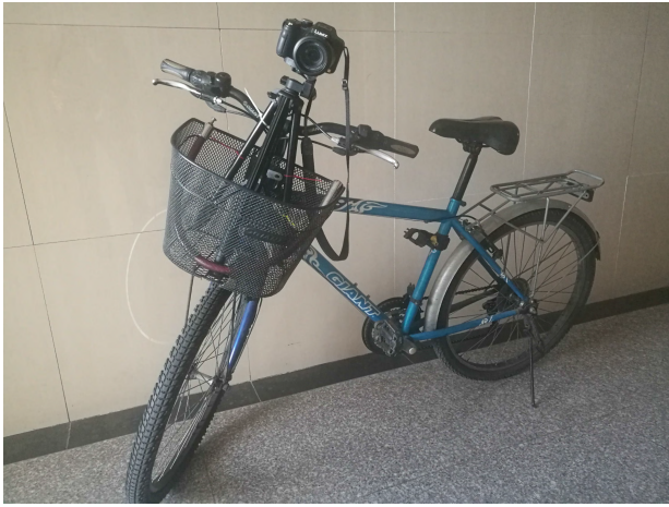
FIGURE 1. The data recording platform: a bike with a common camera.
