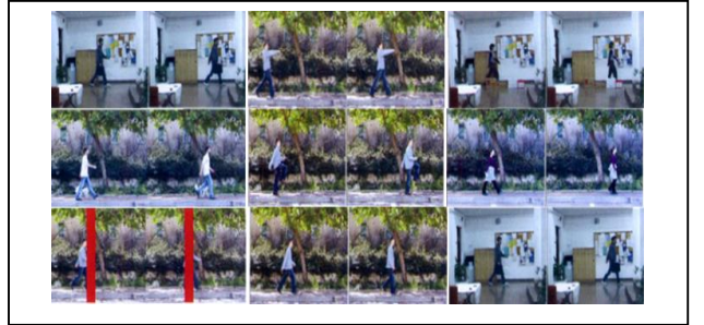
Figure 6. Test walking sequences under different conditions. Rows from top to bottom, lines from left to right are examples of walking with swimming a bag, moonwalk, walking with occluded feet, walking with a dog, walking with knees up, walking in a skirt, walking occluded by a pole, limping walking and walking with a briefcase.
